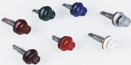
Hex washer head ( powder-painted head in popular colors) self drilling screw, assembled with steel bonded epdm washer
